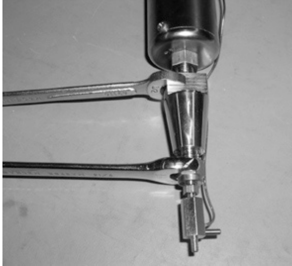
Figure 30 Tightening the Heater Swivel Nut
